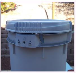
below the lid so it wont pinch the air line. That way you can lift the lid easily without dealing with moving or disconnecting the air lines. I just used the soldering iron to burn the notch down the side
