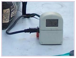
For best results with the timer, make sure it 's rated for 15 amps (usually called heavy duty). I had one that was rated for 10 amps but it burned out in just a few days. The heavy duty (15 amp) timers haven't burned out in over 2 years now.
