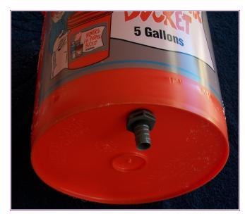
Now that you have the whole cut, insert the through hole and tighten it up. Just make sure you have the rubber gasket on the right side, in most cases (depending on the particular through holes your using) it will most likely be on the outside of the bucket, and only the nut on the inside. In order to keep algae growth down you will need to light proof the buckets. Algae needs two things to grow, food and light. The nutrients will provide plenty of food, so you need to block the light.
