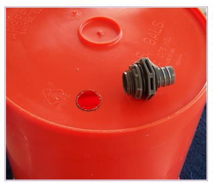
First step is to trace the side of the through hole with the thread and nut, on the bottom of all 4 five gallon buckets. You'll want it to be close to the edge of the bucket, but not so close you wont be able the thread the nut on in order to install it (about an inch). That's so you will be able to set it upright on a table or bench, and most of the buckets weight will still be supported, and it wont tip over.
