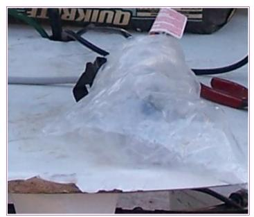
When growing outside, you will want to make sure the timer and cord connections don't get wet or they will short out. This can be done by placing them in a spot that wont get wet even if it's windy and rains hard. In my case I warped 3 plastic bags, layered one on top of the other (in case of small holes). Then tightly duct taped it to the cords. It's not as pretty as it can be, but it kept rain off the connections just fine.
