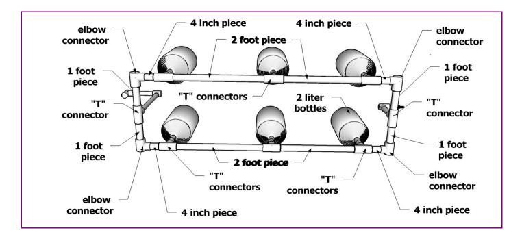
The image below is a top view of the base of the hydroponic system. Notice The short pieces of ¾ inch PVC tubing pointing straight up from each of the "T" connectors where each of the six 2 liter bottles will be placed. Make sure these pieces aren't too long or the 2 liter bottles can become a bit tipsy. Two to three inches should be fine, and again make sure to dry fit everything together first before gluing them together.
