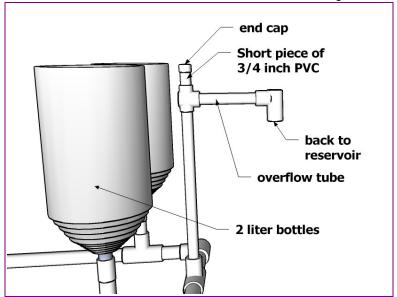
The picture to the left shows the overflow tube going straight down into the reservoir. The reservoir in the picture hasn't been painted yet. But like you did with the 2 liter bottles,
