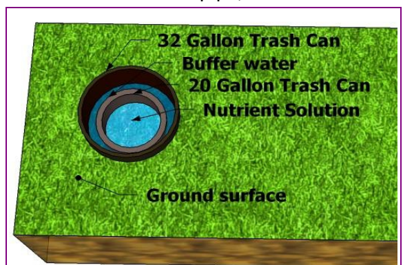
Geothermal Nutrient Reservoir
